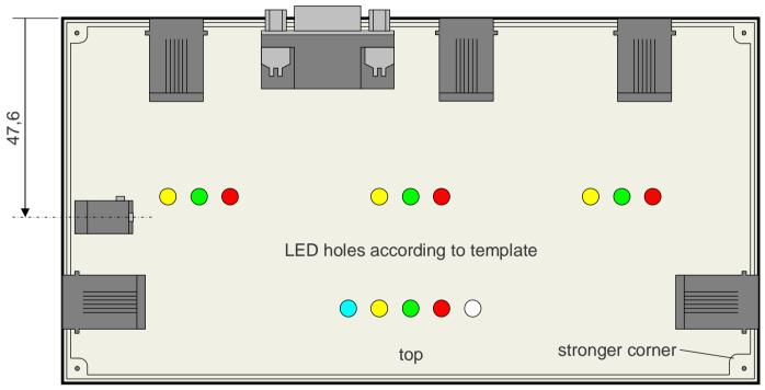
Hole for Low Voltage Power Plug 11mmØ 1,8 mm from outside case edge = 3,0 mm from "top" case edge 3mm Tx- / Rx- / Error-LED3mm Heartbeat-LED3mm Re-connect-LED
